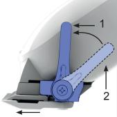
If the clipper has a taper arm, move this back and forth to work the oil through
